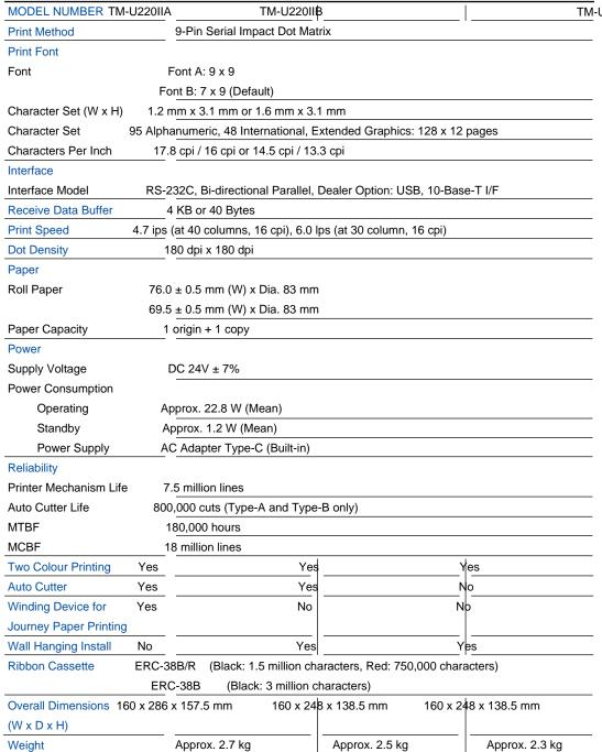
Dimensions & Weight TM-1122011A Weight: Approx. 2.7kg 157.5mm (6.2")286mm (11.26")160mm
